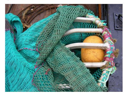
Figure 3: Double flaps (the dark green mesh which is folded back) are used to cover the escape opening; a single large float is used on this TED; there is a mixture of round and square bars in this TED.
