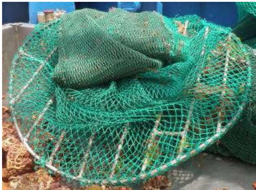
Plate 1: The TED fitted in a trawl net used on the prawn trawl surveys in Kenya and Tanzania in 2011.
